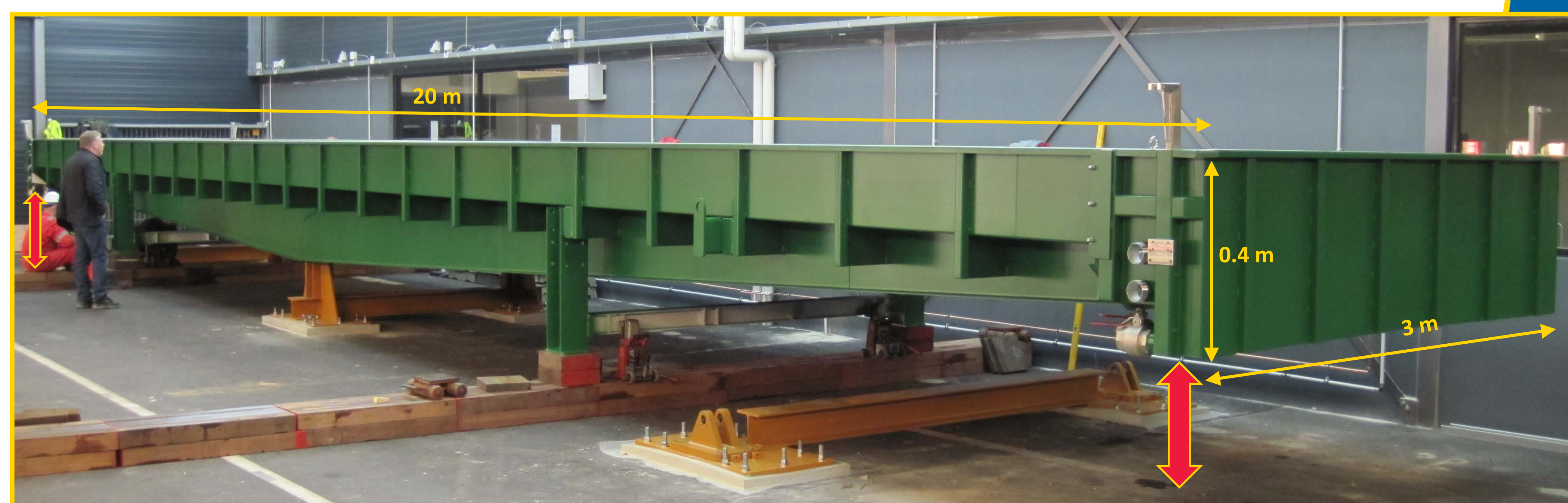
Figure 4. Placing of the 'Metronome', a novel experimental tilting flume to create dynamic tidal systems
